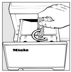
■ Turn the dial to the required setting. Use the spatula supplied with the machine. It is located at the rear of the dispenser drawer facia (see page 23).
